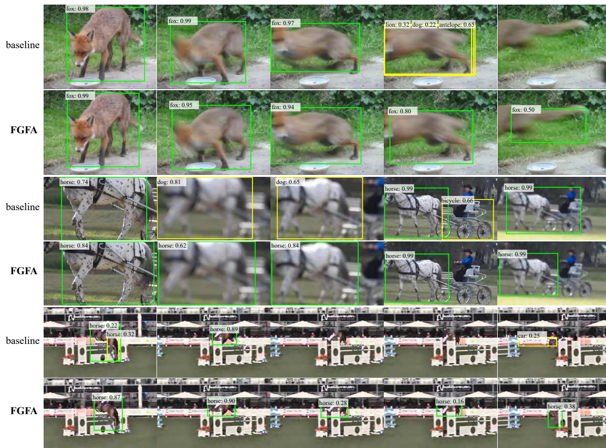
Figure 6. Example video clips where the proposed FGFA method improves over the single-frame baseline (using ResNet-101). The green and yellow boxes denote correct and incorrect detections, respectively. More examples are available at https://youtu.be/R2h3DbTPvVg .
