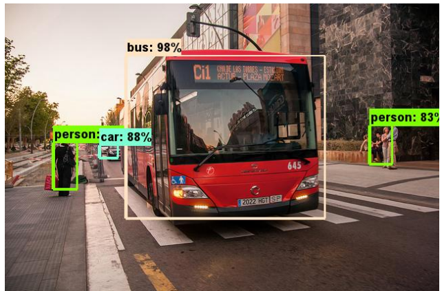
Figure 6. Example objection detection results using MobileNet SSD.
